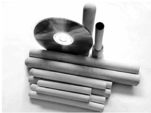
Figure 6. Porous tubular/dead-end tubular supports and CMR obtained by casting technology.
